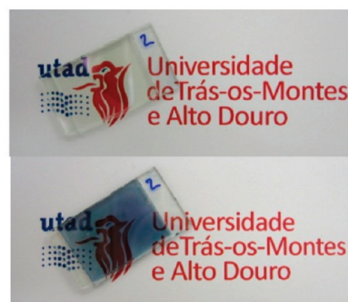
Figure 9. Transmission spectra of the as-deposited (black line), bleached (red line), and colored (blue line, 1st cycle) glass/IZO/ \text{WO}_3 /d-PCL-(530)/siloxane _{6.1}\text{Li}_{12}\text{Eu}_{12} /IZO/glass ECD. The pictures shown below the graphic reproduce the bleached and colored states of this ECD.
